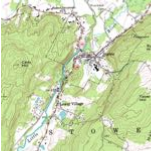
Detailed quantitative representation of land relief using contour lines
